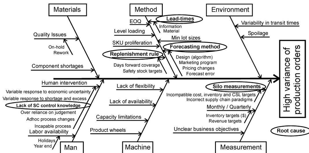
Figure 2. Ishikawa diagram of the causes of the bullwhip effect within Lexmark
