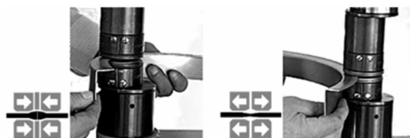
Figure 4: Different directions of bending of angles by shrinking and stretching
