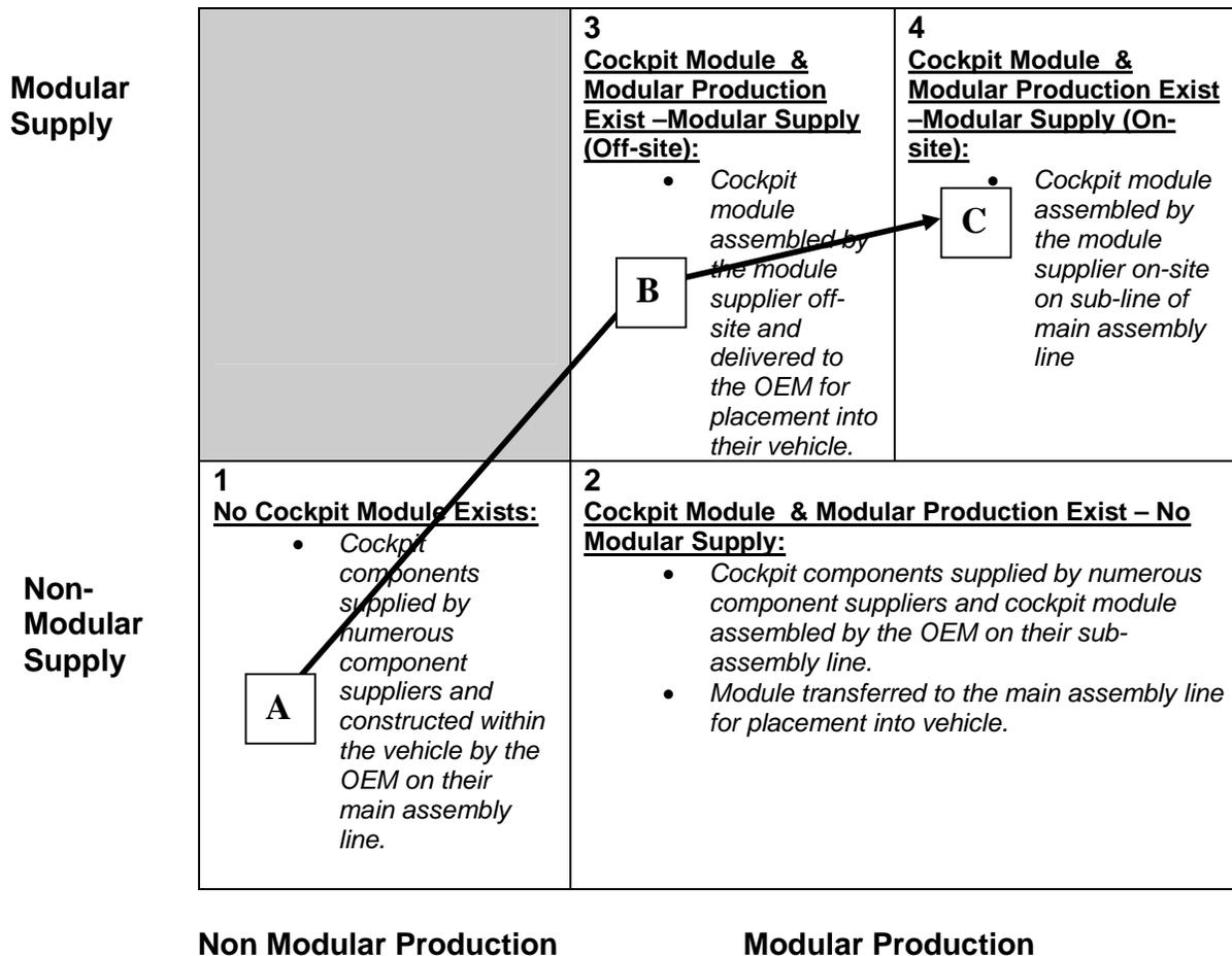
**Figure 2: Cockpit Production and Supply Grid**
