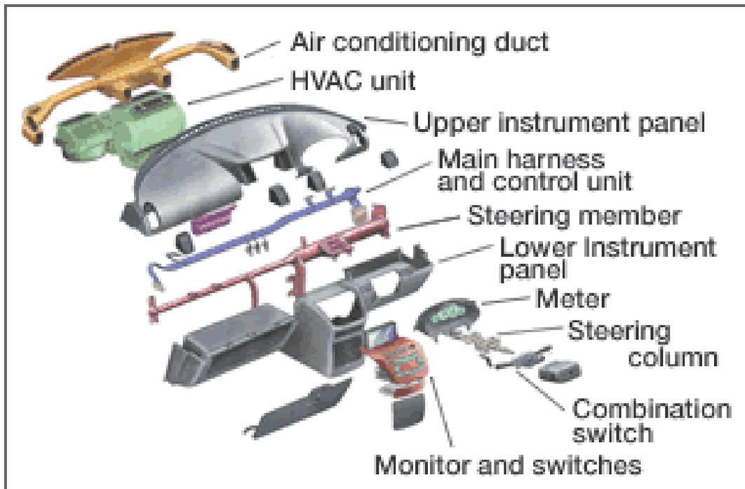
Figure 1. Example of Cockpit Module
