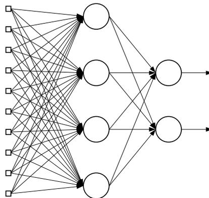
Figure 2: Single layer architecture in a SOM neural network.
