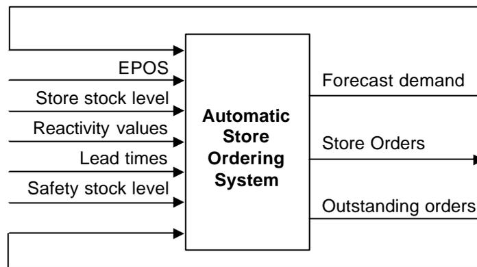
Figure 3. Input-output diagram of Tesco's ASO system
