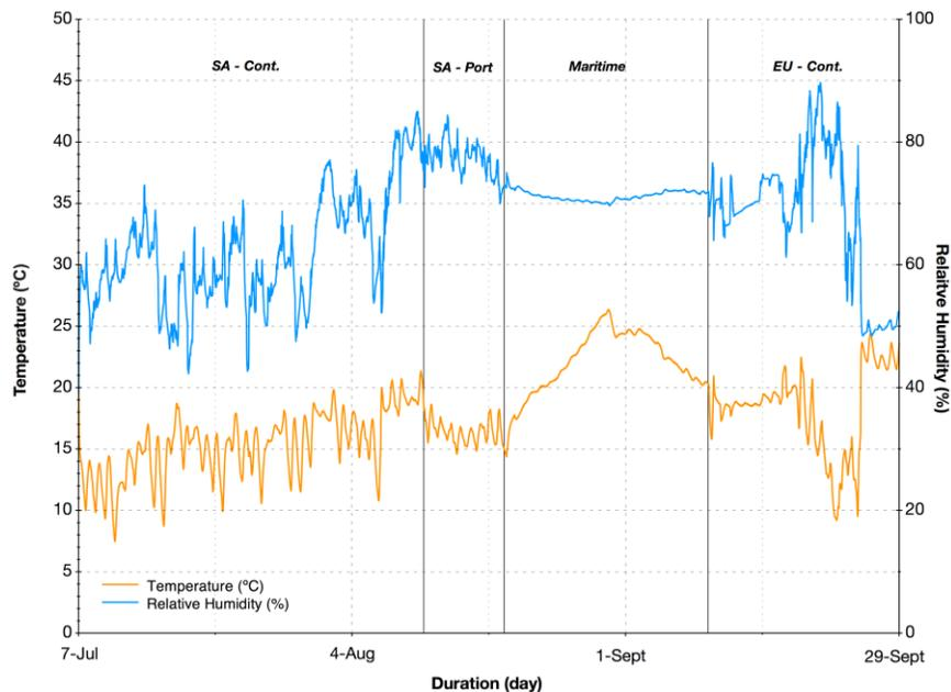
Figure 5 - Temperature and relative humidity (RH) values by timer trigger
