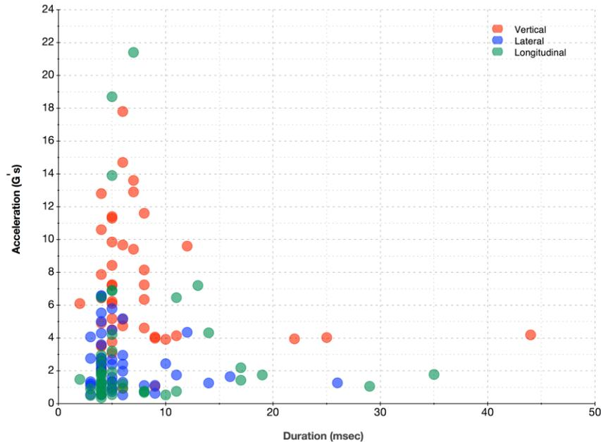
Figure 9 - Recorded shock events in the all three axes with durations
